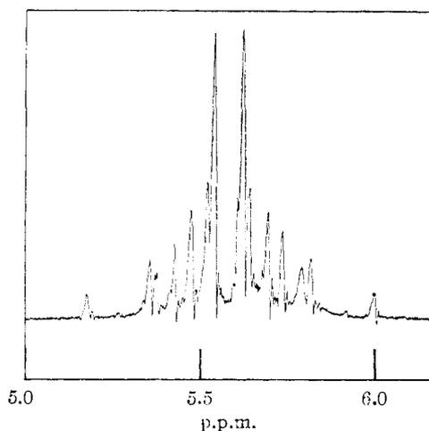
Fig. 1.—P.m.r. spectrum of ethylene sulfite at 40 Mc.p.s. on the scale in which tetramethylsilane as internal standard is at 10.0 p.p.m.<sup>7</sup>
