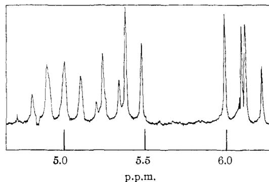
Fig. 4.—P.m.r. spectrum for the ring protons of propylene sulfite isomer ii at 60 Mc.p.s. on the scale in which tetramethylsilane as internal standard is at 10.0 p.p.m.<sup>7</sup>
